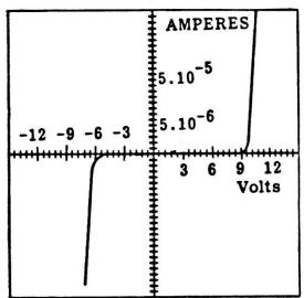
Fig. 3 - Gate-Source I(V) characteristic at  $T = 300^{\circ}K$
