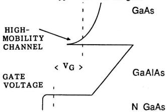
Fig. 2 Energy band diagram when a buried gate voltage V<sub>G</sub> is applied.
