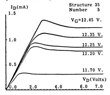
Fig. 4 - Output I<sub>D</sub> - V<sub>D</sub> characteristics for different V<sub>G</sub>
