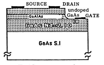
Fig. 1 Structure cross-section.
