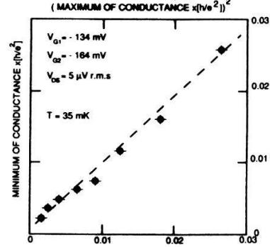
Fig.5 Plot of the conductance minima versus the conductance maxima The experimental points correspond to different values of  $V_{G0}$ .
