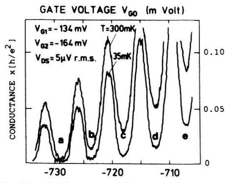
Fig.2 Periodic zero bias conductance oscillations versus  $V_{G0}$  for two temperatures measured at  $\sim 11 \text{ Hz}$
