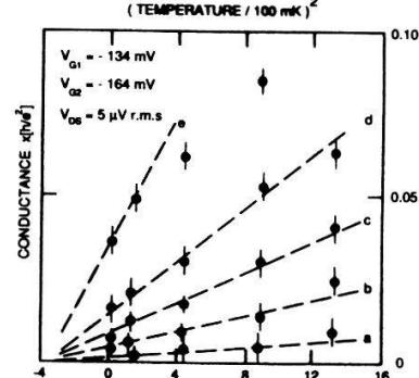
Fig.4 The zero-bias conductance versus  $T^2$  at the minima labelled a – e in Fig.2.
