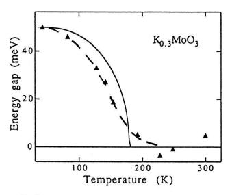
Figure 2: Temperature dependence of the energy gap deduced from photo -emission measurements. The dashed line is a guide for the eye, and the solid line is a BCS curve.
