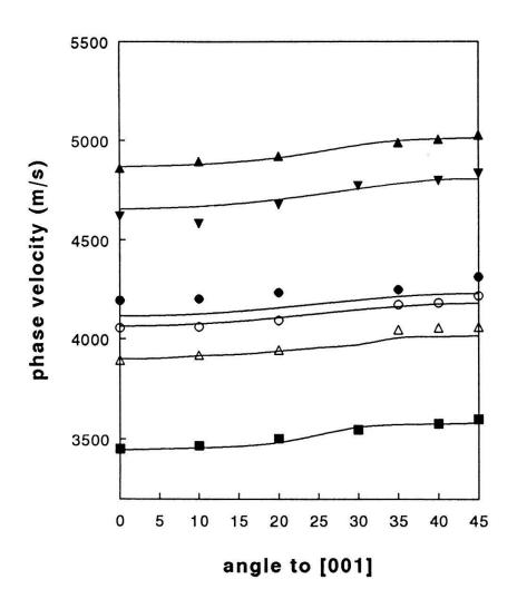
In conclusion, we have compared the measured AD of Si<sub>1-x</sub>Ge<sub>x</sub> with the calculated one using the linearly interpolated elastic constants of the constitutents and found in general good agreement between theory and experiment.
