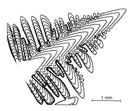
Fig. 1 Contours of a xenon dendrite at 90 s intervals.
