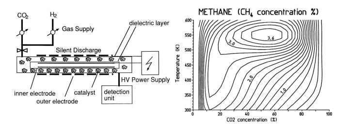
Fig. 1: The experimental set-up
