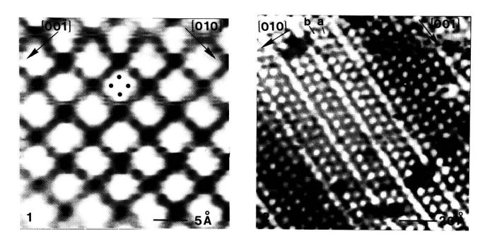
Fig 1:  $(\sqrt{2}x\sqrt{2})R45$  on a Co-rich surface  $(V_{sample} = -5mV, I_t = 40nA)$ Fig.2:  $(3\sqrt{2}x\sqrt{2})R45/(\sqrt{2}x\sqrt{2})R45$  on a Si-rich surface  $(V_{sample} = -10mV, I_t = 4nA)$
