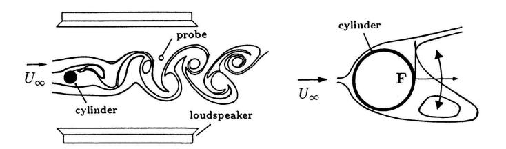
Fig.1: Vortex street with control arrangement Fig.2: Modelling and control via the presused so far
