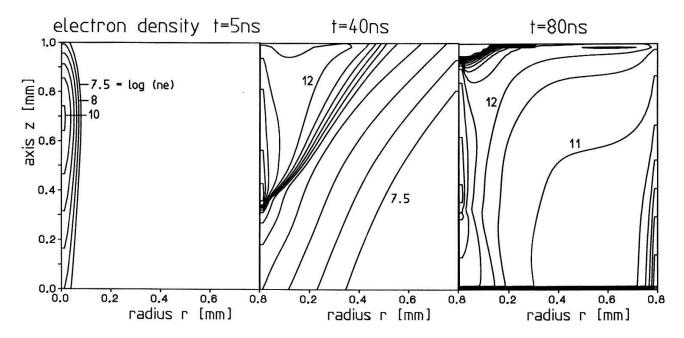
Fig. 1: Electron densities in space at three different times. (Applied field = 160 Td, gap = 1 mm, dielectric thickness = 0.8 mm,  $\varepsilon_r$  = 3)
