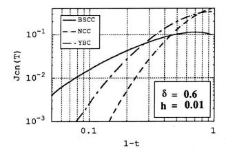
Fig. 1 Temperature dependence of the critical current density for *H* // the basal plane.
