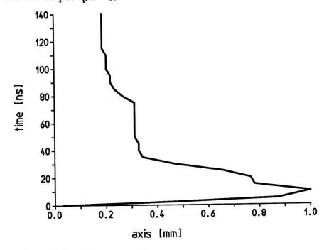
Fig. 2: Location of the electron avalanche front as a function of time. The avalanche is "reflected" at the anode. The front is defined at the 20 % value of max (n<sub>c</sub>).
