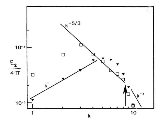
Figure 9. Experimentally observed energy spectra in a two-dimensional turbulence (J. Sommeria, 1986). Arrow indicates the injection wavenumber.
