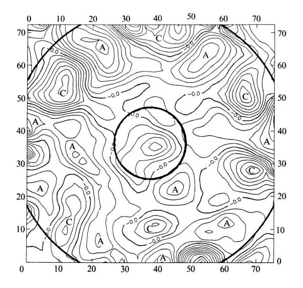
Figure 8. Isovorticity contours on a regular 32<sup>2</sup> grid. Contour levels drawn outside the boundaries of the tank (heavy lines) are artifacts of the contouring routine which insists on data on a rectangular grid. The cyclones are indicated by C, while the anticyclones are indicated by A.
