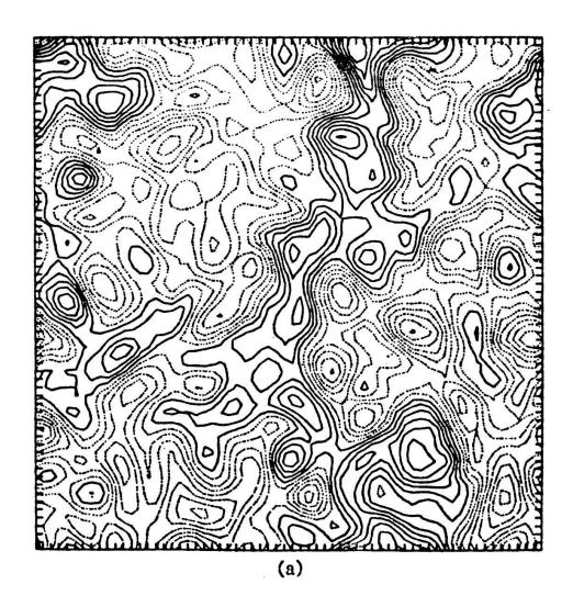
Figure 6. Stream function (a) and vorticity (b) at the 160th time step, t = 10.87, for the wavenumber 8 experiment with  $v = 2.5 \times 10^{-4}$  and  $\tau = 0.5$ , all in dimensionless units.
