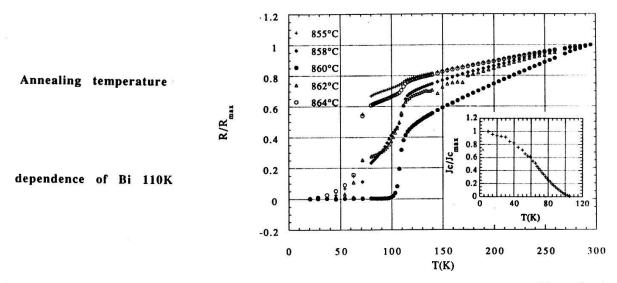
The results show that the loss of the initial Pb concentration in the film during the annealing can be compensated by the sintered ceramic. This element increases and stabilizes the 110 K phase.
