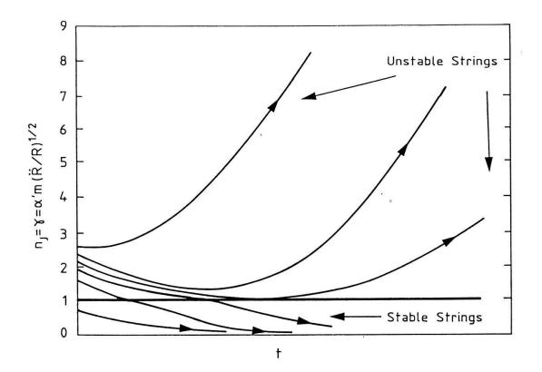
"Bifurcation" in the evolution of strings in an inflationary epoch (with  $\dot{H} < 0$ ). "Unstable" strings manage to stay above  $\gamma = 1$  all the time and blow up. "Stable" strings fall below  $\gamma = 1$  and then stay small forever.
