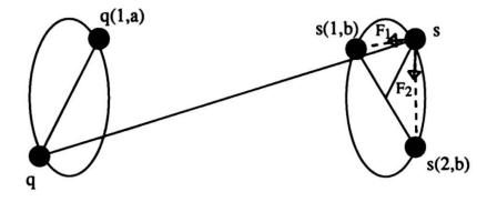
If the force F(1,a) is smaller than the force F(2,a) the particle q will move towards the particle q(2,a)and arrive finally at the point -a of the circle A. The particle s that is still connected with q by means of the rigid rod, will arrive at the point a of the circle B (fig 8).
