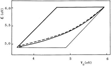
Figure 3 Energy  $\varepsilon$  of the interface state versus the interface potential step  $V_0$  for a variety of heterojunctions with B=1;  $A_{r1}=0.2$ ;  $A_{r,2}=1.5$ ;  $A_{l1}=1.9$ ;  $A_{l2}=1.5$ . The common gap is formed from the second gap of the right-hand crystal and the first gap of the left-hand crystal. Thick straight lines: bottom of the common gap. Full-line curves corresponds to second-type interface states. Dashed-line curve corresponds to first-type interface states.
