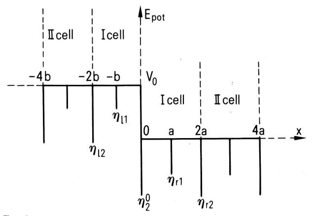
Figure 1 One-dimensional model of the second-type heterojunction between two diatomic semiconductors  $(\eta_{12} = \eta_{r2})$ .
