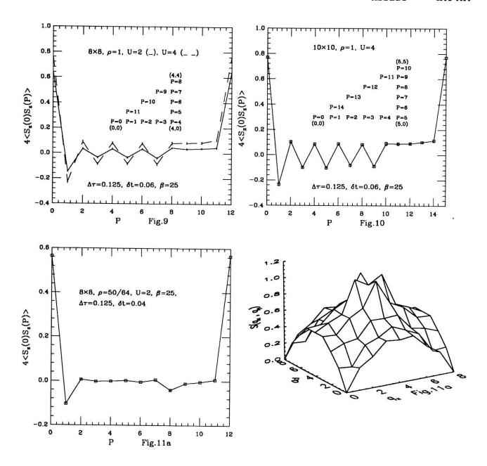
Fig. 9 Spin-spin correlation function for a  $8 \times 8$  lattice at  $\rho = 1$ ,  $\beta = 25$ , U = 2 and U = 4. The numbering denotes the path on the two dimensional lattice: starting at (0,0), going along the x-axis, then along the y-axis and diagonally back.
