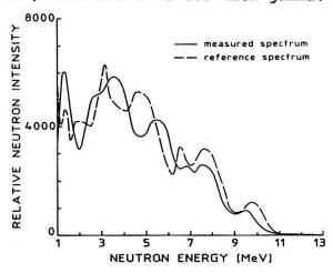
Fig.1: unfolded spectrum PuBe source with NE-230 spectrometer
