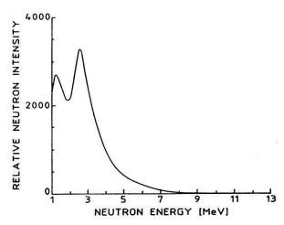
Fig.2: unfolded spectrum <sup>252</sup>Cf source with NE-230 spectrometer
