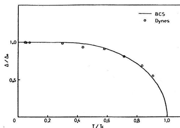
Fig. 2 Temperature dependence of energy gap for  $\text{YBa}_2\text{Cu}_3\text{O}_{7-\delta}$ . A solid line is the BCS characteristic, and a circle the experimental value.
