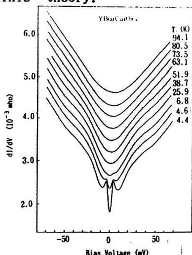
Fig. 1  $V$ - $dI/dV$  characteristics of  $\text{Pb-SiO-YBa}_2\text{Cu}_3\text{O}_{7-\delta}$  junction at temperatures ranging over from 4.4 to 94.1 K.
