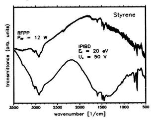
Fig. 2: IR spectra of an IPIBD film ( $E_I=20eV$ ,  $U_A=50V$ ) and RFPP film ( $P_{rf}=12W$ ).
