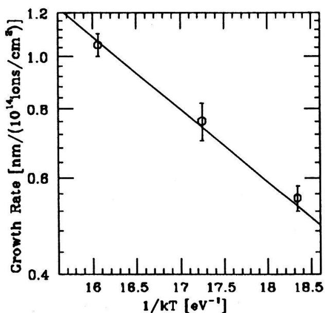
Fig. 3. Growth rate as a function of  $1/kT$ . The growth rate is defined as  $dr/d\phi$ , where  $r$  is the average grain radius and  $\phi$  is the Kr dose.
