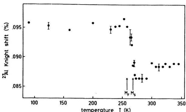
**Fig. 1 :** Temperature dependence of the  $^{27}\text{Al}$  Knight shift.
