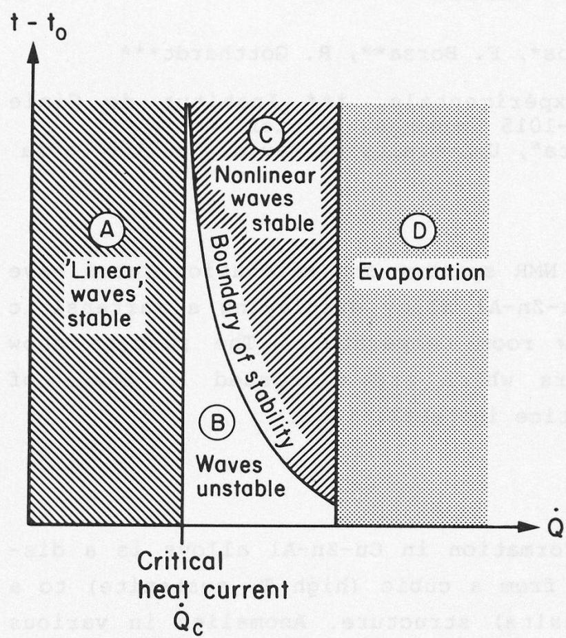
Fig. 1 - The time  $(t - t_0)$  after switching on the wave generator as a function of the heat current  $\dot{Q}$ .
