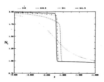
electronic transition is driven by the strength of the Coulomb interaction between c and f-electrons: increasing the value of G from 0 to 1.5 eV the transition passes continuously from second order to first order.
