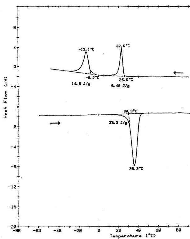
Fig.2-Cooling and heating DSC scans for a specimen aged at 500 C.
