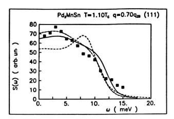
Fig. 2 Experimental data [7] for the Heusler compound  $Pd_2MnSn$  at  $T=1.1~T_c$  and  $q=0.7q_{ZB}$  in the (111) direction are shown together with results from theoretical calculations. The solid and dash-dot curves are mode coupling calculations with six and eight shells of neighbours, respectively, and the dashed curve is the theoretical three pole approximation. Calculated spectra are convoluted with a resolution function.
