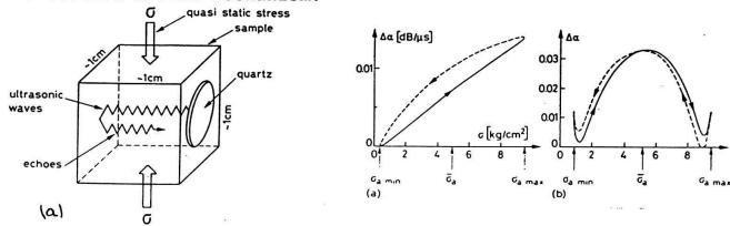
Fig. 3 (a). The principle of the measurement device using the two-wave acoustic coupling method; (b) Two examples of signature obtained in 5-N aluminium.
