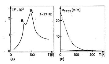
Fig. 1. (a) The Bordoni peak measured in 6N aluminium; (b) the critical resolved shear stress measured in pure aluminium. The dotted line represents the value of  $\sigma_{\text{CRSS}}$  which is theoretically expected from the Bordoni peak measurement.
