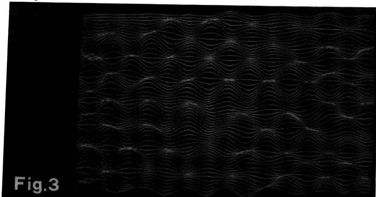
Pure TAPO solution on a similar gold substrate can be imaged only in the constant-current mode and appears as a crystalline structure of centered hexagons of 3.1 Å side. Fig.3 is a constant-current image (25 Å by 25 Å) of TAPO molecules in amplitude-trace representation as it appears on the computer during data acquisition. The absence of imaging in the barrier-height mode is probably due to a negligible modification of the work function of gold by TAPO.
