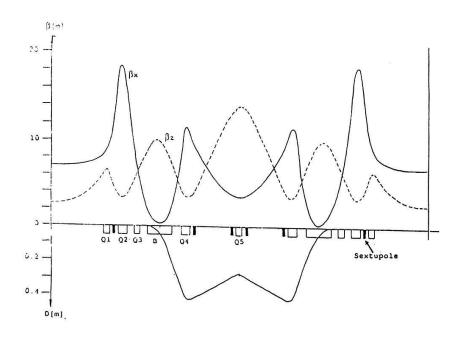
Fig. 3 Achromat structure and lattice functions.
