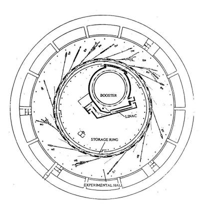
Fig. 2 Layout of the linac, booster, storage ring and experimental hall.
