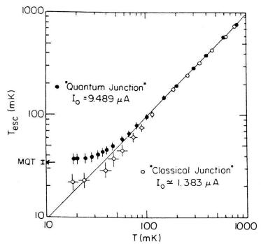
Figure 8 Escape temperature plotted against temperature for two values of the critical current. The solid line is the classical prediction  $T_{\rm esc} = 0.95 \, {\rm T}$  (equation (8)). The arrow is the quantum prediction (equation (10)).
