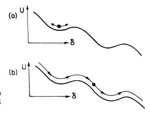
Figure 2 The two states of a Josephson junction biased with a current  $I < I_0$ ; a)  $\langle \dot{\delta} \rangle = 0$  (zero voltage state); b)  $\langle \dot{\delta} \rangle \neq 0$  (voltage state)
