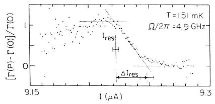
Figure 5 Microwave induced enhancement of the escape rate measured as a function of the bias current.  $\Omega/2\pi$  is the irradiation frequency.
