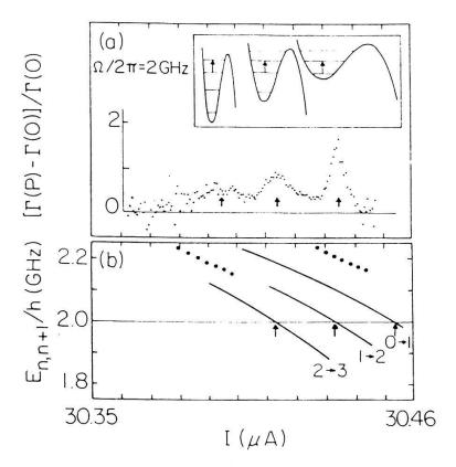
Figure 7 a) Microwave induced enhancement of the escape rate as function of bias current for  $k_BT/\hbar\omega_p=0.29$ . Arrows indicate positions of resonances. Inset represents the corresponding transitions between energy levels. b) Calculated energy level spacings. Dotted lines indicate uncertainties in  $E_{01}$  due to errors in the determination of junction parameters. Arrows indicate values of bias current at which resonances are predicted.
