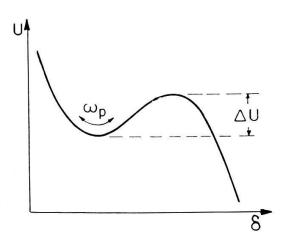
Figure 4 Cubic potential from which the particle representing the junction phase difference escapes.
