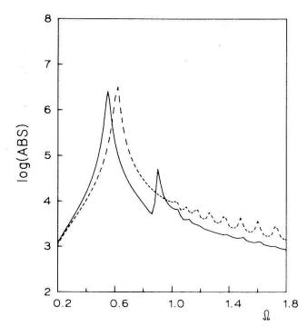
Figure 1 Absorption curve of a sphere of radius R = 20 Å with a linear density profile and surface diffuseness  $r_o = 4 \text{ Å}$ . The broken curve gives the sharp surface results for comparison. Absorption is in arbitary units and  $\Omega = \omega/\omega_p$ .
