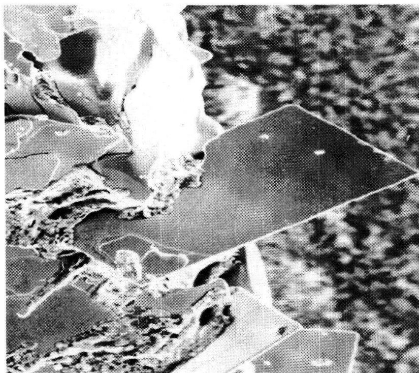
Figure 2 SEM picture of a \text{YBa}_2\text{Cu}_3\text{O}_{7-x} tiny plates which has grown on a copper oxide needle (size 100 \times 70 \mu\text{m}^2 , thickness about 1–3 \mu\text{m} ).
