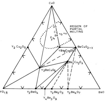
Figure 1 YO<sub>1.5</sub>-BaO-CuO quasi-ternary phase diagram [12] between 950 and 1000°C.
