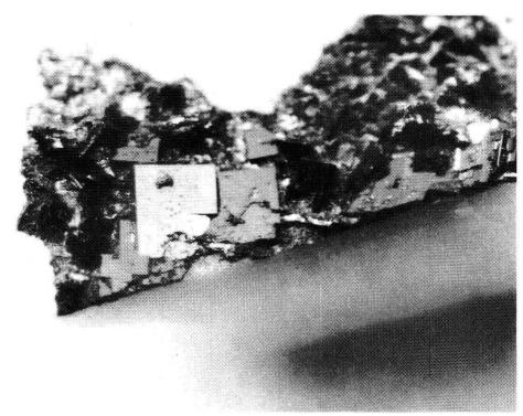
Figure 5 Photograph of  $YBa_2Cu_3O_{7-x}$  (up to  $2 \times 2 \times 0.3$  mm<sup>3</sup>) which have grown above the separate liquid.
