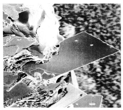
Figure 2 SEM picture of a YB<sub>2</sub>Cu<sub>3</sub>O<sub>7-x</sub> tiny plates which has grown on a copper oxide needle (size  $100 \times 70 \,\mu\text{m}^2$ , thickness about 1-3  $\mu$ m).
