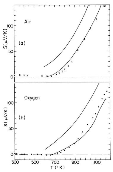
Figure 1 The temperature dependence of the TEP in YBaCuO in air (a) and in oxygen at 1 bar (b). The measured values are shown by points and crosses; the range of values calculated by equation (1), using  $\delta(T)$  taken from the different reports in Ref. 2, is shown by continuous lines.
