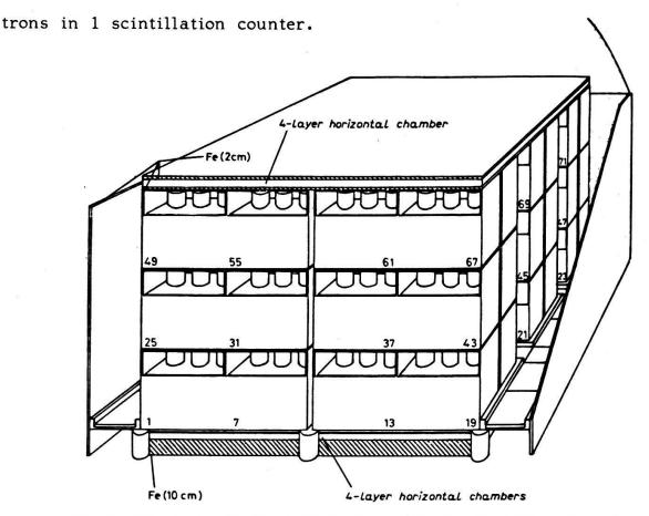
Fig. 1. - The 90 ton liquid scintillation detector in the Mont Blanc Laboratory (dimensions  $(7 \times 8 \times 5)$  m<sup>3</sup>).
