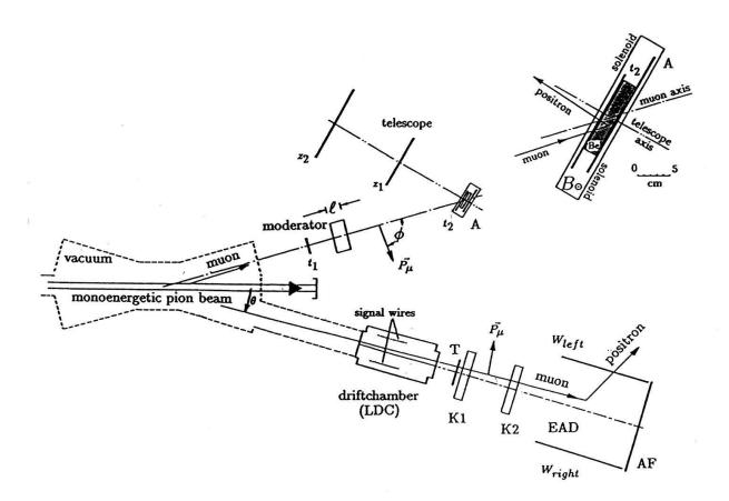
Fig. 1: Apparatus to measure the asymmetry of the directional distribution of positrons from the decay of polarized muons. The transversely polarized muons were extracted at 15.2° from a parallel  $\pi$ -beam. The two approaches to observe the  $\mu$ -decay are shown:
