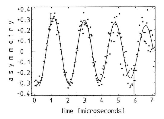
Fig. 4: Measured time distribution between the muon stop in Be and the observation of the decay positron, based on about 100000 events. The exponential  $\mu$  decay time has been divided out. The solid line is  $A(t_{\mu})$ . The fit yields the desired value of  $P_{\mu}\xi$  as  $C/(1-\epsilon)$ . (The slow decrease in amplitude (relaxation) is due to internal fields in Be).
