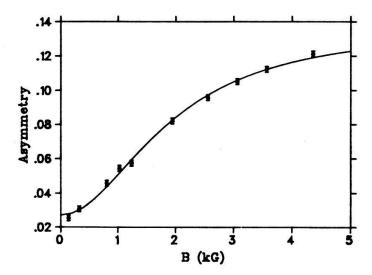
Fig. 2 Asymmetry vs longitudinal field strength for muonium in KCl. The circles refer to a recent measurement by Gygax et al.<sup>5</sup> performed at room temperature. The solid line represents the fit to these data using our model on muonium relaxation. The parameter values are the same as those of Fig. 1:  $\tau_c = 1.9 \times 10^{-10} s$ ,  $\delta_{ex} = 60$  MHz, and  $\tau_R = 0.5 \times 10^{-6} s$ .
