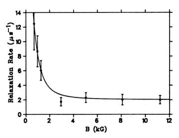
Fig. 1 Transverse relaxation rate vs field for muonium iin KCl at room temperature. The circles refer to a recent measurement by Baumeler et al..<sup>6</sup> The solid line was obtained solving our model on Mu depolarization with  $\tau_c = 1.9 \times 10^{-10} s$ ,  $\delta_{ex} = 60$  MHz, and  $\tau_R = 0.5 \times 10^{-6} s$ .
