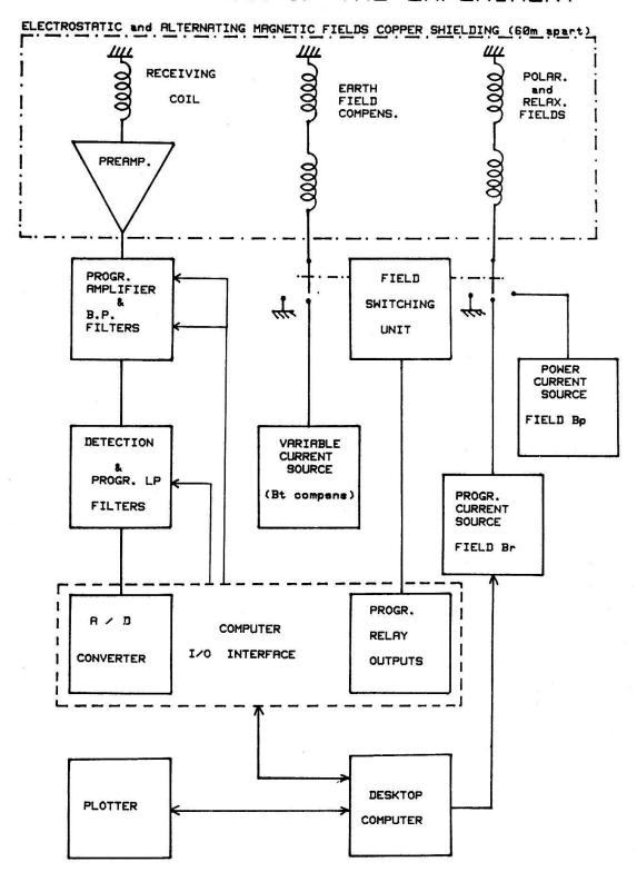
Figure 3 Block diagram of the experiment.
