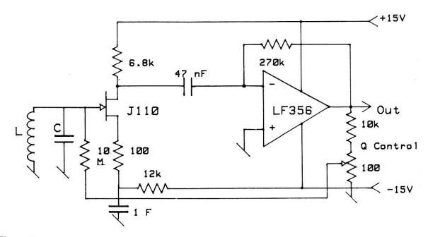
Figure 6 Low noise and high input impedance preamplifier, the regeneration loop controls the coil Q. Gain from 1500 to 30 000 (depending on the Q control), input noise voltage from 1.5 nV/ $\sqrt{\text{Hz}}$  at 200 k $\Omega$  input impedance to 4 nV/ $\sqrt{\text{Hz}}$  at 2 M $\Omega$  impedance (high Q).
