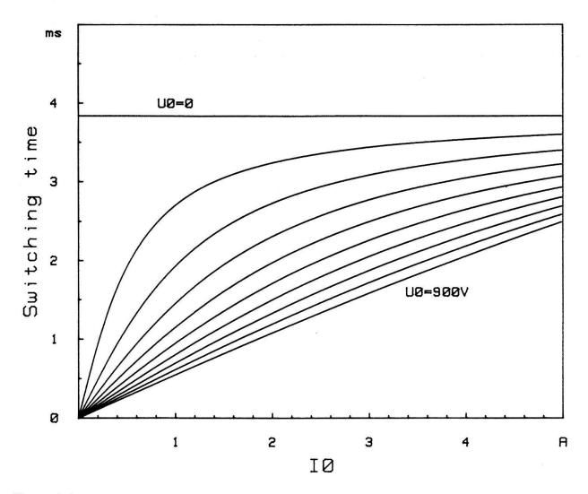
Figure A.1 Switching time for the capacitor circuit, if the capacitor value is the optimum one at  $I_0 = 5$  A. With no precharging voltage, switching time is independent of the current,  $\tau = \pi/2\omega$ .
