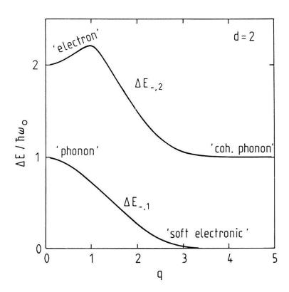
Figure 2 Energy of the first two  $\sigma' = -\frac{1}{2}$  excited states, measured from the ground state energy  $E_{+1}$ , as a function of the vibronic coupling  $q = \lambda/\hbar\omega_0$  for d = 2.0. The character of the modes changes with q, as described in the text.
