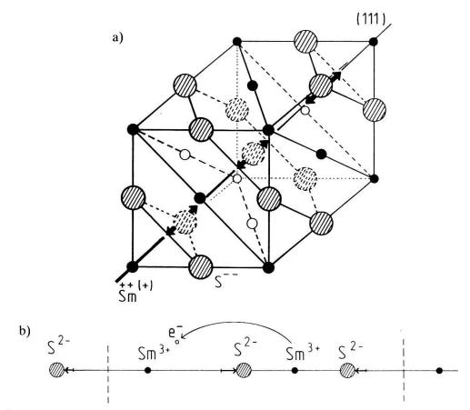
Figure 1 Vibration of the  $S^{--}$  planes in the longitudinal  $q = \pi/a(111)$  mode for the NaCl-type SmS (or  $Sm_xY_{1-x}S$ ) lattice. The small filled circles are metal ions, the anions (big circles) oscillate along the (111) direction; a) the elementary cube (elongated on the drawing, to point out the planes in phase); b) the equivalent linear chain.
