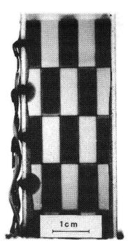
Figure 3 Display based on the aluminum suspension. The fluid depth is  $1.0\,\mathrm{mm}$ . In the transparent areas a voltage of  $\pm 30\,\mathrm{V}$  is applied.
