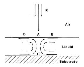
Figure 2 A thin liquid layer, illuminated by the radiation R. The IR absorbing region A is heated and a convection flow starts. Small plates in the liquid align horizontally in the area B and vertically at A.
