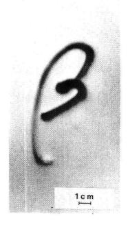
Figure 5 The effect of static charging on the suspension. The letter  $\beta$  has been written with a synthetic brush.
