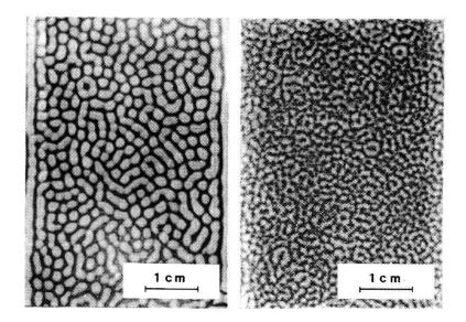
Figure 1 Convection induced by an instable density distribution, performed in a thin (2 mm) fluid cavity. (a) The case of Rayleigh convection, (b) The case of sedimentation.
