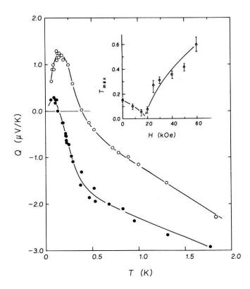
Fig. 4: Thermoelectric power of two samples of CeAl<sub>3</sub>. Insert: field dependence of the temperature maximum of Q.
