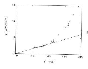
Fig. 6: Thermal conductivity of of UBe $_{13}$  far below its superconducting transition  $T_c$  0.9 K. Dashed line: linear temperature  $\alpha T$  dependence of  $\kappa$ .
