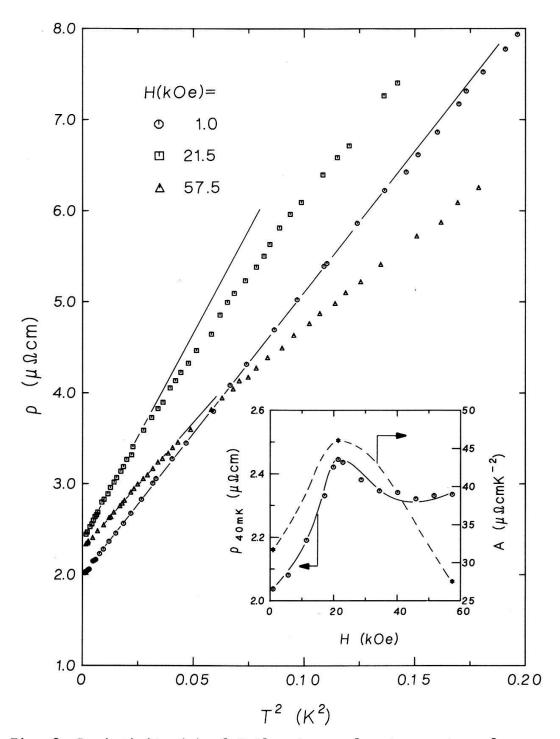
Fig. 2: Resistivity ( $\rho$ ) of CeAl $_3$  at very low temperature for three different fields. Insert : field variation of the residual resistivity  $\rho_0$  and of the A coefficient of the resistivity law :  $\rho(H) = \rho_0 + AT^2$ .
