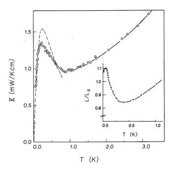
Fig. 3: Thermal conductivity of CeAl<sub>3</sub> as a function of the temperature.
