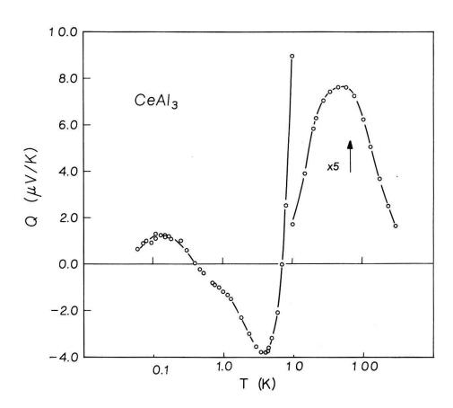
Fig. 1: Thermoelectric power Q of CeAl<sub>3</sub> over almost 4 decades of temperatures.
