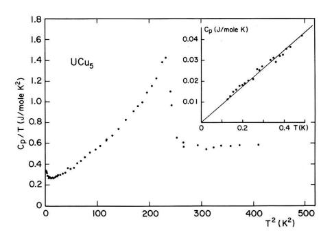
Figure 16 - Low-temperature specific heat of UCu<sub>5</sub> between 0.15 and 21 K.
