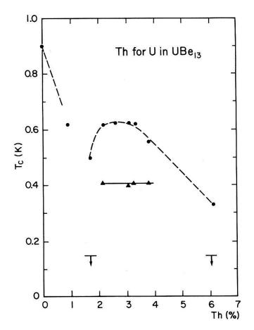
Figure 12 Critical temperatures for  $U_{1-x}^{\rm Th}_{\rm X}^{\rm Be}_{13}$  from c<sub>p</sub> measurements. Dots indicate the superconducting transition, triangles the second transition at  $T_{\rm c2}$ . At 1.7 and 6% Th, no second transition was observed above 0.15 K.
