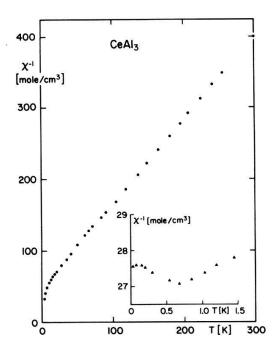
Figure 2  $\chi^{-1}(T)$  of CeAl<sub>3</sub>. Data between 4.2 and 300 K are from ref. [6], data below 1.5 are from ref. [3].
