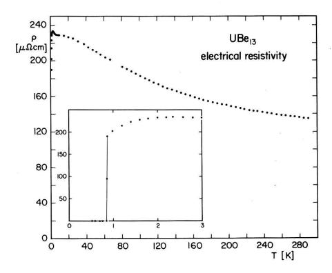
Figure 4 -  $\rho(T)$  for UBe<sub>13</sub> between 1.2 and 300 K. The inset shows the super-conducting transition on an extended temperature scale.
