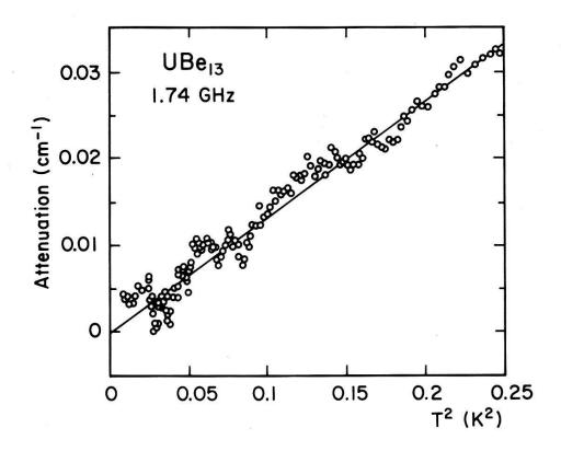
Figure 8 - Temperature dependence of the attenuation of ultra-sound in superconducting UBe $_{13}$  between 0.1 and 0.5 K.
