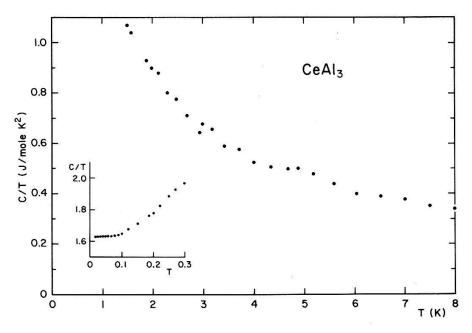
Figure 3 -  $c_p/T$  versus T for CeAl $_3$  at low temperatures. The data for T < 0.3 K are from ref. [3].
