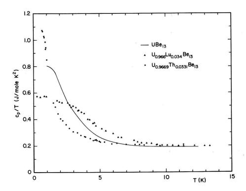
Figure 11 - Comparison of the influence of different impurities on the lowtemperature normal-state specific heat of UBe<sub>13</sub>.
