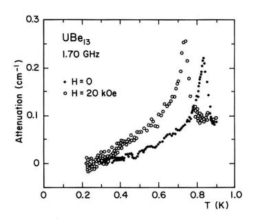
Figure 9 Accoustic attentuation peak in superconducting  $UBe_{13}$  below  $T_{c}$  The peak shifts to lower temperatures with increasing magnetic field.
