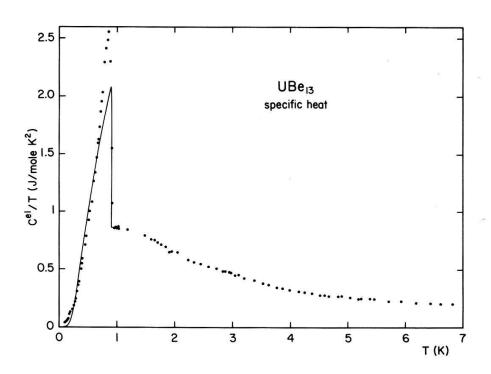
Figure 5 - Electronic specific heat of UBe $_{13}$  plotted as  $c_p^{el}/T$  versus T between 0.15 and 7 K. The solid line marks the prediction of the BCS-theory.
