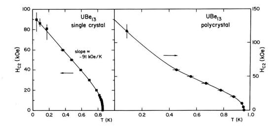
Figure 6 -  $H_{c2}(T)$  for single-crystalline and polycrystalline UBe $_{13}$ . Data are from ref. [14].
