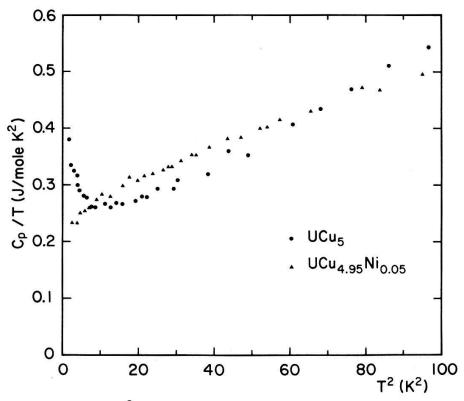
Figure 18 - c/T versus  ${\rm T}^2$  for UCu<sub>5</sub> and UCu<sub>4</sub>  $_{95}{\rm Ni}_{0}$   $_{05}$  between 1.5 and 10 K.
