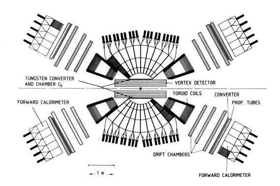
Fig. 6 Schematic cross section of the UA2 detector in the vertical plane containing the beam.
