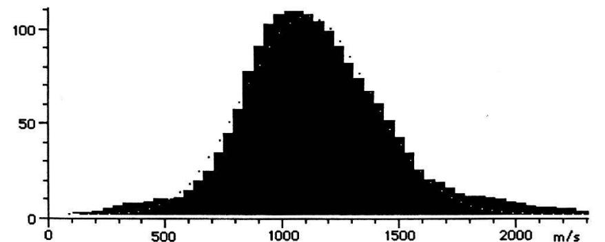
$V_{\text{drift}} = 858 \text{ m/s}$   $T = 11.1 \text{ K}$   $V_{\text{max}} = 1035 \text{ m/s}$  Mach number = 2.7
