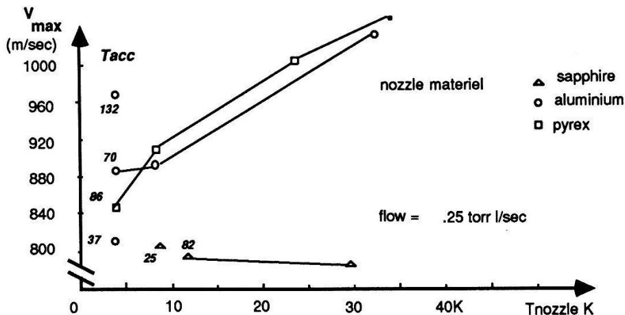
Tacc = temperature of the accommodator (geometry b)
