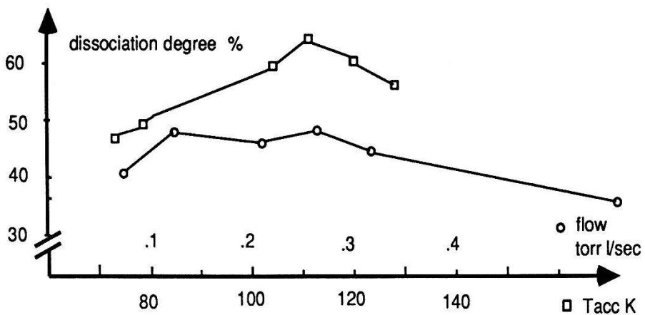
Fig. 6 Dissociation degree (geometry fig 2 b , nozzle material: sapphire)
