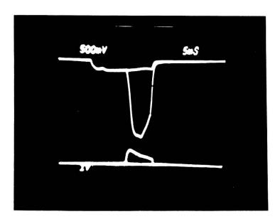
Figure 3 - The upper trace shows H produced by resonant charge exchange (10  $\mu A/V$ ). The lower trace shows the H signal from the hydrogen dissociator.
