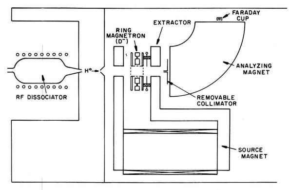
Figure 2 - Experimental setup for measuring the H production.
