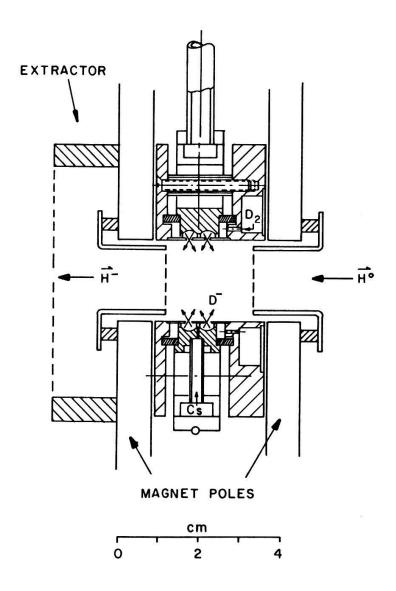
Figure 1 - Schematic of the ring magnetron ionizer.
