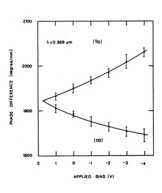
Fig. 3 Phase difference between TE and and TM modes as a function of the applied bias for the two orthogonal light propagation directions along [110] and [T10].
