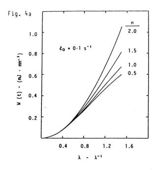
Absorbed energy per unit volume for different strain parameters
