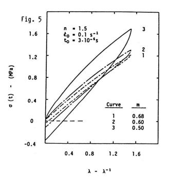
Dissipated energy per unit volume for various strain parameters
