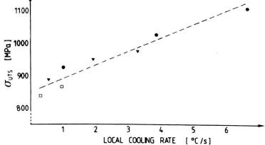
Figure 8 Tensile strength and tensile elongation of Ni-19% Cr-0.46% C alloys as a function of the cooling rate.
