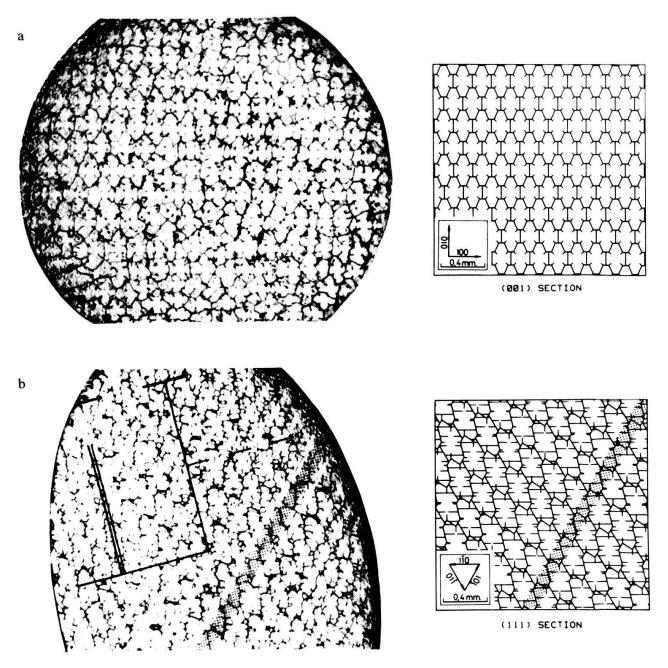
Figure 10 Comparison between real and computed sections of dendritic single crystals. Upper row (a): (001) crystallographic sections. Lower row (b): (111) crystallographic sections.
