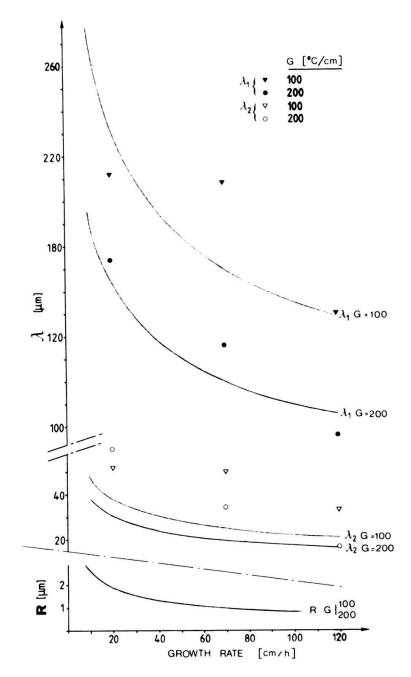
Figure 4 Comparison between measured and calculated values of dendrite spacings  $\lambda_1$ ,  $\lambda_2$  and tip radius R as a function of the growth rate v.
