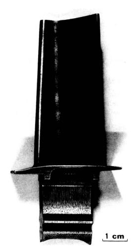
Figure 2 Monocrystalline turbine blade for aircraft application. Such turbine blades are made from Nibase superalloys using a modified Bridgeman crystal growth technique.
