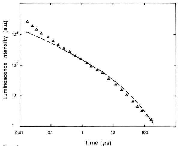
Figure 2 Total photoluminescence intensity vs. time.  $\triangle$ : Experimental decay following a pulsed excitation. Undoped a-Si:H, excitation energy 2.31 eV, excitation density  $6 \times 10^{-7}$  J cm<sup>-2</sup>. Temperature 77 K. --: Theoretical decay as predicted by our model.
