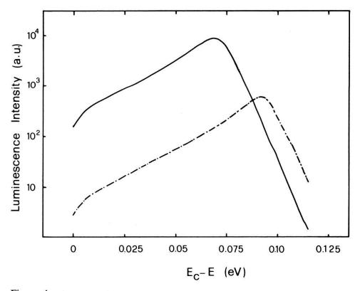
Figure 4 Photoluminescence intensity as a function of energy for —:  $t_1 = 0.1 \,\mu\text{s}$ , — · —:  $t_2 = 10 \,\mu\text{s}$ .
