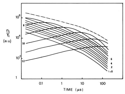
Figure 3 Contributions to the photoluminescence emission from the different energy intervals with energies  $E_i = i \cdot 0.012 \text{ eV}$  below the mobility edge. i = 0 corresponds to contributions from the mobility edge with  $E_0 = 0$ . —: total photoluminescence intensity.
