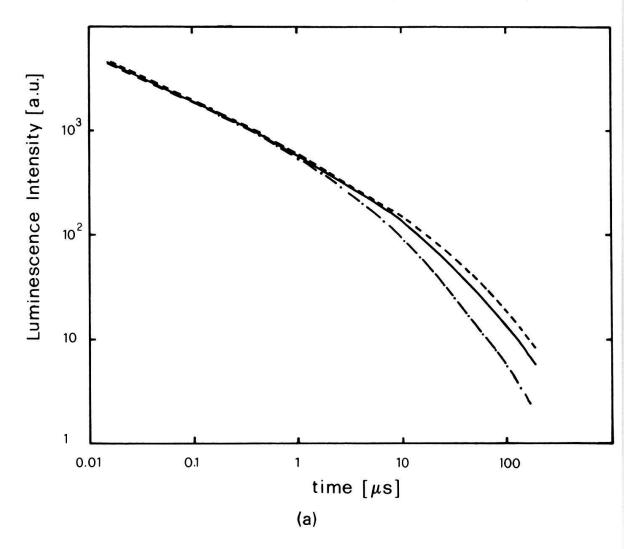
Figure 5 Total photoluminescence intensity vs. time for different temperatures.
