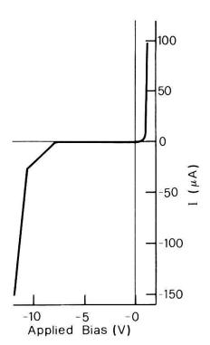
Figure 2 Current-voltage characteristic of the MQW device.
