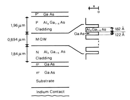
Figure 1 Schematic of the MQW structure. The insert schematically shows the Al concentration x to vary from x = 0 to x = 0.24.
