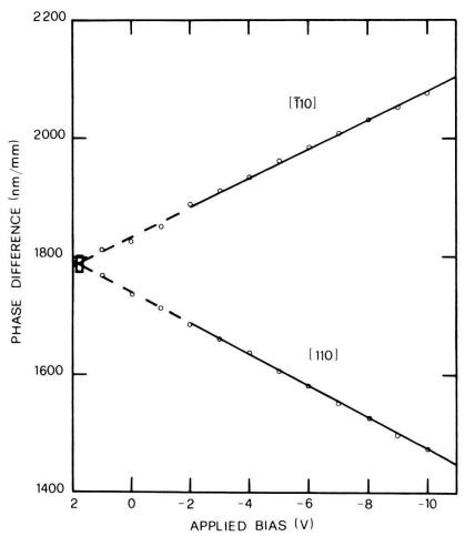
Figure 4 Phase difference between TE and TM modes as a function of the aplied bias for the two orthogonal light propagation directions along [110] and [110]. The solid lines are linear fits to the data for  $V_a < -2 \text{ V}$ . Their extensions for  $V_a > 2 \text{ V}$  are dashed.
