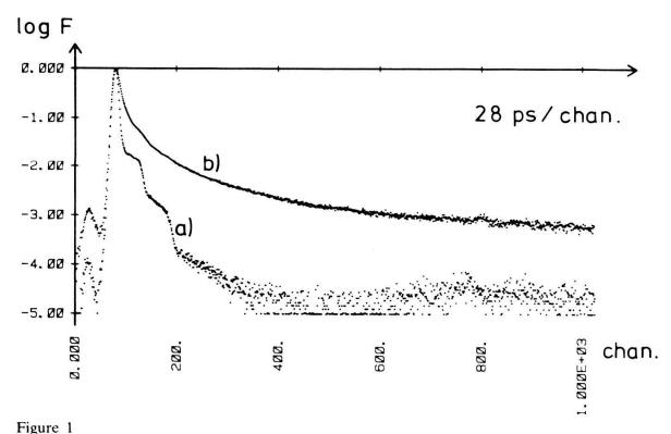
(a) Response of our measuring system to 5-ps-pulses of the dye laser. (b) Fluorescence decay of a tetracene crystal with a magnetic field of 0.5T in the direction of the a-axis (off resonance). Excitation at 300 nm, observation at 546 nm, temperature:  $62^{\circ}$ C.
