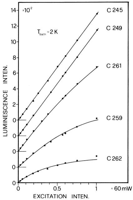
Figure 4 Integrated iodine luminescence intensity (arbitr. units) in the system AgBr: I as a function of excitation intensity. Fit of the corrected data to equation (8). Per sample there are two fitting points.
