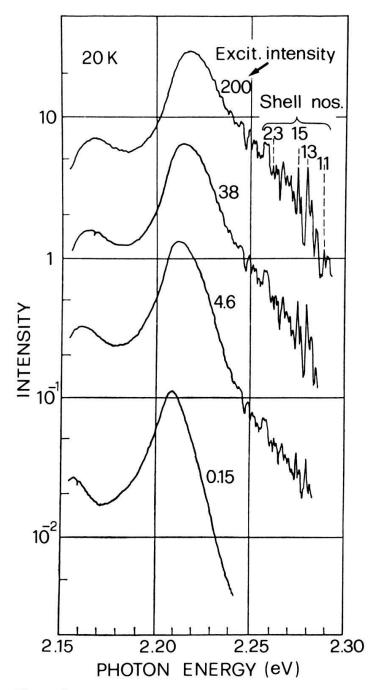
Figure 1 Donor Acceptor Pair Spectra in the system GaP:S, C at different excitation intensities, from Ref. 4.
