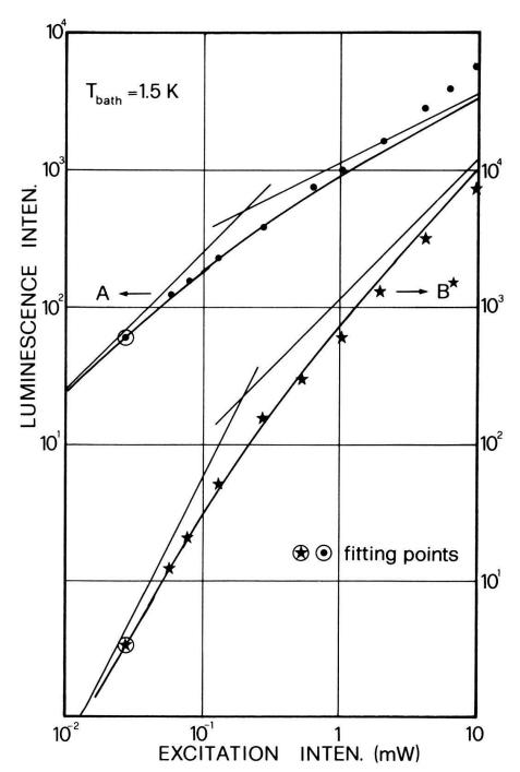
Figure 2 Bound exciton and bound biexciton luminescence intensity in GaP:N as a function of excitation intensity. A fit to the solutions equation (5) of the rate equations is shown. Note that the two pairs of asymptotes intersect at the same excitation intensity. Parameter values:  $J_0 = 0.05 \text{ mW}$ , P = 249, Q = 58.5.
