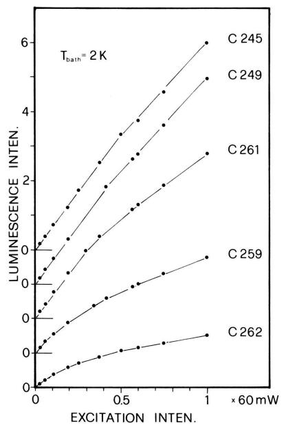
Figure 3 Integrated iodine luminescence intensity (arbitr. units) in the system AgBr: I as a function of excitation intensity. The points correspond to the raw experimental data. The lines connecting the points are guides to the eye.
