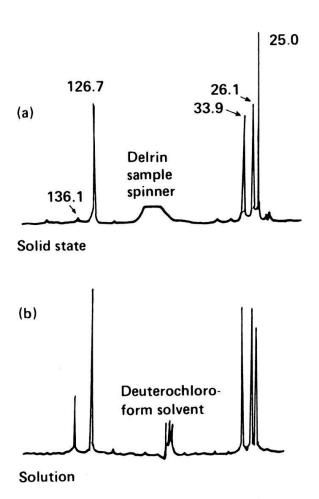
Fig. 7. (a)  $^{13}$ C NMR spectrum of solid vulcanized polyisoprene (b)  $^{13}$ C NMR spectrum of unvulcanized polyisoprene in deuterochloroform solution.
