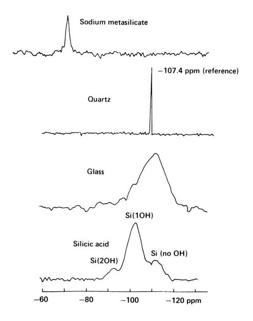
Fig. 2. Typical  $^{29}\mathrm{Si}$  NMR spectra of some common silicious materials
