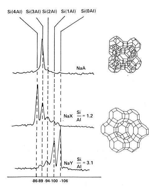
Fig. 4. Effect of Si/Al ratio on the  $^{29}\mathrm{Si}$  spectra of synthetic zeolites.
