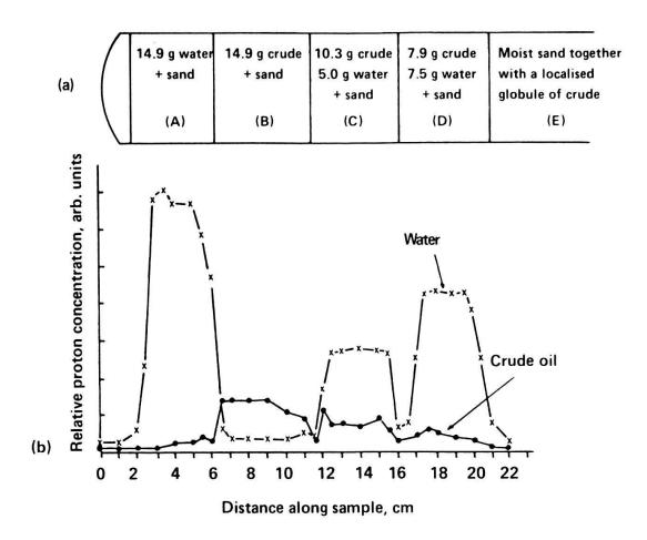
Fig. 8. Composition (a) and measured proton concentrations (b) of crude oil and water in a simulated core sample.
