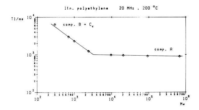
Fig. 6: Molecular weight dependence of the proton spin-lattice relaxation times of linear polyethylene. The plateau ( $M_{\rm W} > M_{\rm AB}$ ) is governed by component A. At low molecular weights the common influence of components B and  $C_{\rm C}$  is visible.
