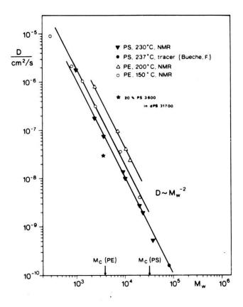
Fig. 2: Molecular weight dependence of (weight average) center of mass self-diffusion coefficients in polymer melts (linear polyethylene (PE) and atactic polystyrene (PS)) measured by a NMR field-gradient technique [15]. For  $M_{\rm W} < M_{\rm C}$  the molecular weight dependence of the free volume enters as revealed by the reduced diffusion coefficient of PS 3600 in a matrix of deuterated PS 31700.
