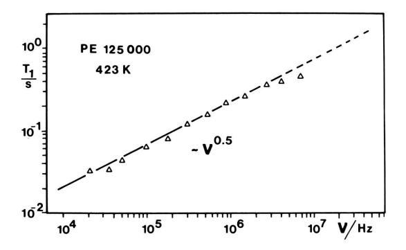
Fig. 3: Frequency dependence of the proton spin-lattice relaxation time of linear polyethylene. The experimental conditions are such that component B dominates (see section 5).
