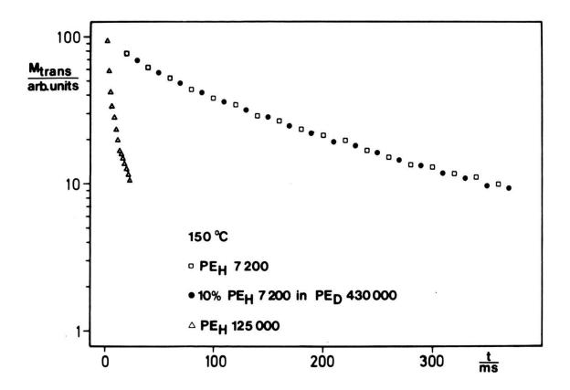
Fig. 4: Transverse proton relaxation curves for PE 7200 pure and dissolved in a matrix of deuterated high molecular weight chains. In order to indicate the sensitivity of the technique, data for pure PE 125000 are also plotted.
