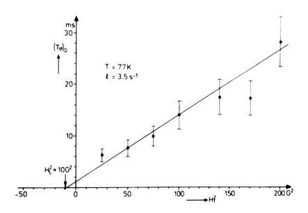
Fig. 6. Plot of the dislocation-induced contribution to the relaxation time T  $_{1\rho}$  vs the locking field H  $_1^2$  of  $^{27}{\rm Al}$  at a constant strain rate  $\dot{\epsilon}$  at 77 K.
