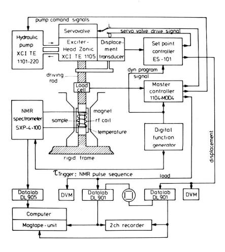
Fig. 2. Block diagram of the experimental set-up.
