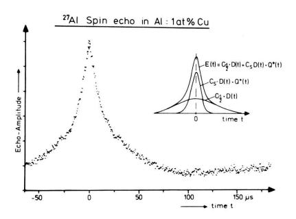
Fig. 5.  $^{27}$ A1 spin echo in Al:1 at.% Cu at 77K. For I=5/2 C and C  $_{\rm S}$ Q  $^{+}$ (t)=0.469 Q(2t)+0.284 Q(4t), see equation 9a.
