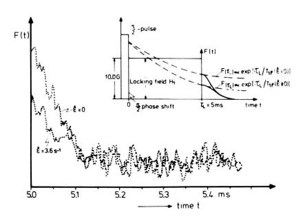
Fig. 4. Result of an in situ NMR tensile experiment showing the  $^{27}$ Al free induction decays F(t) in aluminum after a spin-locking sequence with zero and finite plastic strain rate  $\dot{\epsilon}$ . From the measurement  $T_{1\rho}(\dot{\epsilon}=0)=25.0$  ms and  $T_{1\rho}(\dot{\epsilon}=3.6~\text{s}^{-1})=7.2$  ms is obtained.
