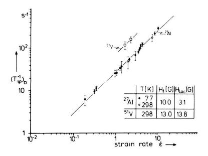
Fig. 7. Dislocation-induced part of the  $^{27}$  Al and  $^{51}$  V relaxation rates (T  $_{1\rho}^{-1}$ ) in aluminium and vanadium as a function of  $\dot{\epsilon}$  for different temperatures D  $(\epsilon \gtrsim 7\%)$ .
