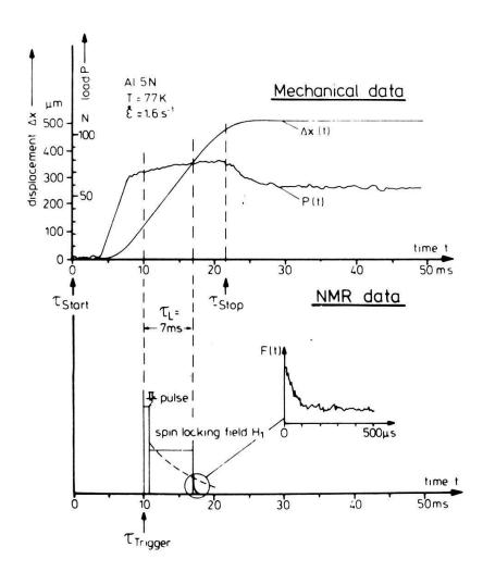
Fig. 3. Displacement  $\Delta x$ , load P, rf-pulse sequence ( $\pi/2$  pulse followed by a locking field of strength  $H_1$ ), and  $^{27}Al$  free inducting decay signal F(t) as a function of time during an in situ NMR tensile experiment on an aluminium foil (see text).
