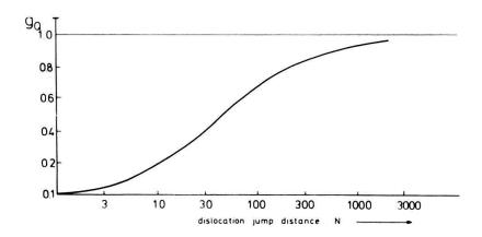
Fig. 1. Quadrupolar geometry factor  $g_{Q}$  for a mobile dislocation as a function of the normalized jump distance N (in units of the Burgers vector).
