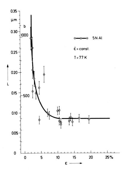
Fig. 8. The mean jump distance measured by NMR as a function of stirain  $\varepsilon$  in Al.
