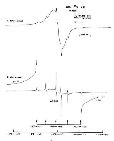
Fig. 6. EPR powder spectra of  ${\rm Fe}^{3}$  in LuPO $_4$ . a) after coprecipitation in molten urea and calcination at 800  $^{\rm O}$ C; b) after annealing in a torch and quenching.
