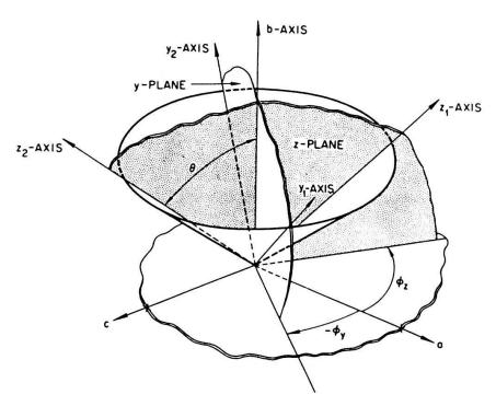
Fig. 10. Orientation of the crystal-field principal axes of  $\mathrm{Gd}^{3+}$  in monazite-type rare-earth orthophosphates. The z- and y-axis for sites (1-4) and (2-3) lie on the same cone (e.g.  $\theta=61^{\circ}$  for  $\mathrm{LaPO_4}\colon\mathrm{Gd}^{3+}$ , Fig. 9).
