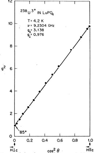
Fig. 12. Position of the U  $^3$  EPR transition in xenotime-type LuPO $_4$ . The square of the g-value is plotted versus  $\cos^2\theta$ , where  $\theta$  is the angle between  $\hat{H}$  and the c-axis.
