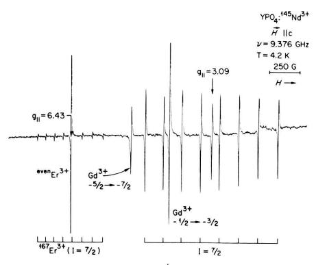
Fig. 13. EPR spectrum of enriched  $^{1+5}Nd^{3+}$  isotopes in xenotime single-crystal. The 8 hyperfine lines corresponding to the various values of  $M_{\overline{I}}$  (I = 7/2) are almost centered around the central g = 3.09 line of the even isotopes. Additional lines of  $Gd^{3+}$  and  $Er^{3+}$  are also labeled.
