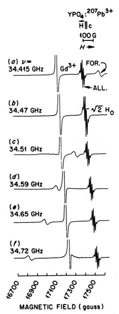
Fig. 3. High-field EPR transitions of 207Pb3+ in xenotime. As the microwave frequency is increased from a to f, the allowed transition moves at higher fields while the forbidden line position decreases.
