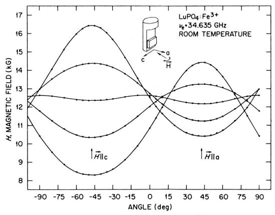
Fig. 5. Angular variation of the 5 EPR lines of  $Fe^{3^{\top}}$  in LuPO. Spectra in Figs. 4a and 4b correspond to the orientation labeled with H c and H a. The powder spectrum shown in Fig. 4c can be obtained by a proper average of this angular variation.
