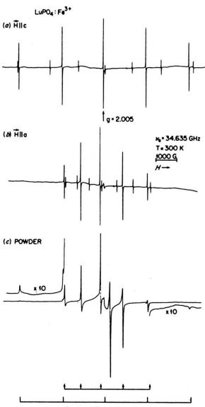
Fig. 4. EPR spectrum of  $Fe^{3^+}$  (3d<sup>5</sup>, <sup>6</sup>S<sub>2</sub>) in LuPO<sub>4</sub>. a) Single-crystal with H c; b) single-crystal with H c and c) powder spectrum. Shoulders and divergences are labeled with sticks and arrows, respectively.
