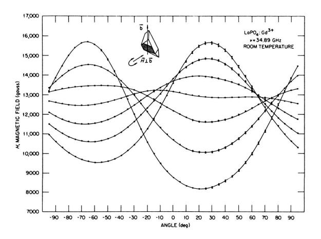
Fig. 8. Angular dependence of the EPR spectrum of Gd<sup>3+</sup> in monazite-type LaPO single crystal with the magnetic field rotated in the plane perpendicular to the b-axis. Each curve is doubly degenerate in this plane.
