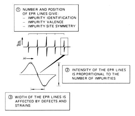
Fig. 14. The type of information provided by EPR.
