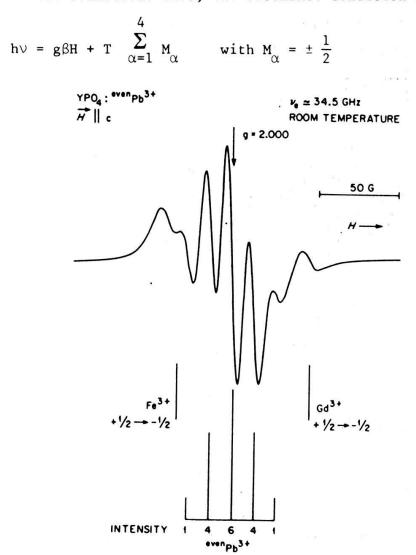
Fig. 1.  $-\frac{1}{2} - +\frac{1}{2}$  EPR transition of even Pb<sup>3+</sup> isotopes in a xenotime single-crystal. The magnetic field is parallel to the c-axis.
