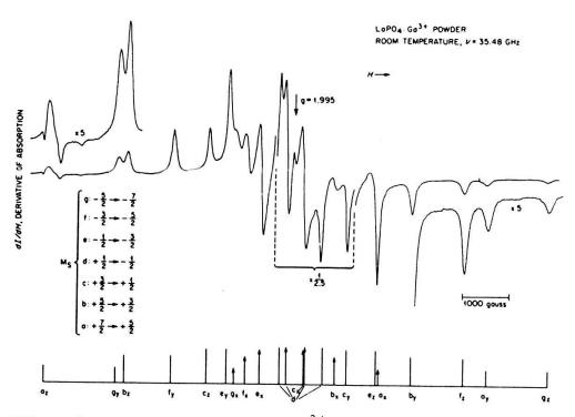
Fig. 11. EPR powder spectrum of LaPO<sub>4</sub>:  $Gd^{3+}$ . Shoulders and divergences are labeled for each transition noted (a) - (g) with sticks and arrows. The central transition  $-\frac{1}{2} \longleftrightarrow +\frac{1}{2}$  has a complicated lineshape due to second-order terms (18).
