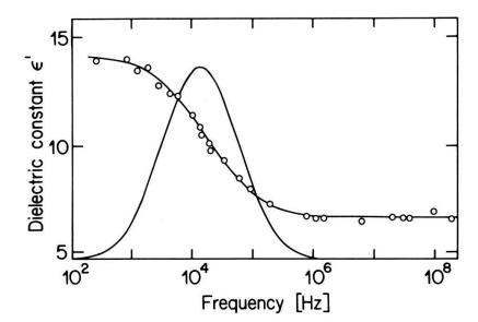
Figure 7 Frequency dependence of the dielectric constant in  $(CH_3)_3NDCdCl_3$  at 297 K with the electric field parallel to the a-axis. (a) The solid line shows the unsatisfactory fit of equation (5) to the data. (b) Fit of equation (7) to the data. The Gaussian is a plot of equation (6).
