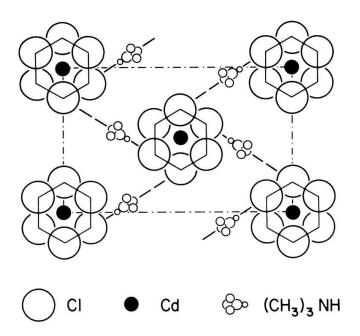
Figure 1 Structure of  $(CH_3)_3HNCdCl_3$  at room temperature, projection along the c axis showing only part of  $CdCl_6$  octahedra. Hydrogen bonds are indicated by dashed lines.
