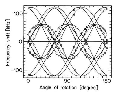
Figure 4 Shift of the deuteron NMR signals in  $(CH_3)_3NDCdCl_3$  with respect to the Larmor frequency for a rotation around the *c*-axis. The zero of the angle of rotation is arbitrary. Solid lines are fits of equation (3) to the data. (a) Pattern at 320 K together with the spectrum at 158°. (b) Pattern at 366 K.
