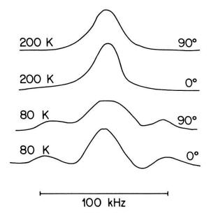
Figure 2 Proton NMR signal in a (CH<sub>3</sub>)<sub>3</sub>HNCdCl<sub>3</sub> single crystal at 80 K and 200 K with the c-axis perpendicular to the magnetic field and two arbitrary orientations of the a-axis differing by 90°.
