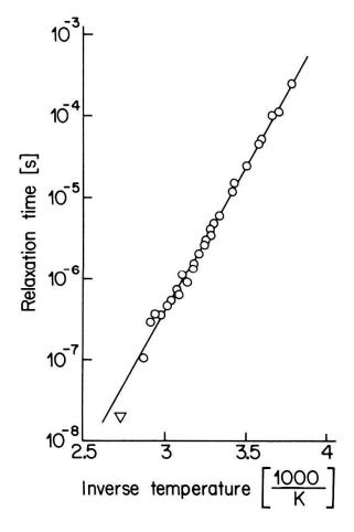
Figure 8 Temperature dependence of the mean-field dielectric relaxation time as defined by equation (8) in  $(CH_3)_3NDCdCl_3$ .  $\nabla$  denotes the value obtained from deuteron NMR relaxation.
