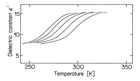
Figure 6 Temperature dependence of the dielectric constant in  $(CH_3)_3NDCdCl_3$  at 0.7, 1.5, 3, 6, and 12 kHz (from left to right). The electric field is parallel to the a-axis.
