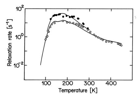
Figure 3 Temperature dependence of the proton relaxation rate in (CH<sub>3</sub>)<sub>3</sub>NDCdCl<sub>3</sub> powder at 32 MHz (full circles) and 90 MHz (open circles). The lines represent a fit of equation (1) to the data.
