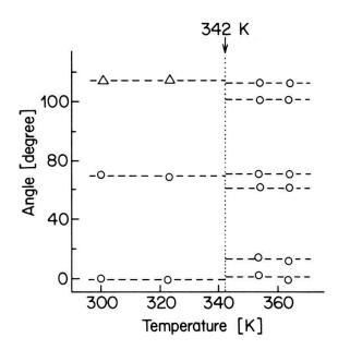
Figure 5 Orientation of the  $V_{zz}$  component of the electric field gradient at the deuteron site with respect to an arbitrary direction in the ab plane in  $(CH_3)_3NDCdCl_3$ .  $\bigcirc$ : observed in all specimens,  $\triangle$ : observed in only some of the samples investigated.
