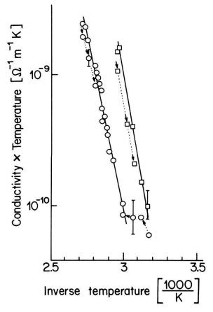
Figure 9 Conductivity×temperature as a function of inverse temperature in  $(CH_3)_3NHCdCl_3$  for the electric field parallel to the c-axis. The arrows denote the sequence of the measurements.  $\bigcirc$  and  $\square$  refer to two different samples.
