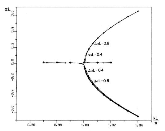
Figure 2 Threshold gain  $\alpha L$  and resonance frequency  $kL = (\omega/c)\bar{n}L$  of a finite DFB structure with M = 100 periods, length L. Rectangular gain modulation with  $\Delta \alpha L$  growing in steps of 0.2 and uniform index n = 1.5.
