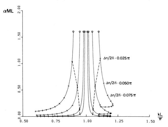
Figure 1 Threshold gain  $\alpha ML$  and resonance frequency  $kL = (\omega/c)\bar{n}L$  of a finite DFB structure with M = 100 periods, length L, for the resonances with  $N - M = \pm 1$ ,  $\pm 2$ ,  $\pm 5$ ,  $\pm 10$  in the case of rectangular index modulation with average index  $\bar{n} = 1.5$  and modulation strength  $\Delta n/2\bar{n}$  growing in steps of  $0.1 \cdot \pi/4$ .
