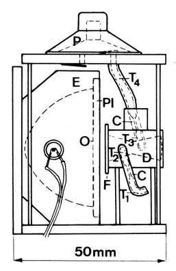
Figure 1 Photoacoustic gas detecting device. The light source is thermally modulated.
