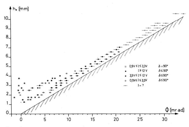
Figure 3 Resonances as functions of grating angle  $\phi$  and waveguide height  $h_0$  (see Fig. 1). I indicates pulse energy expressed in V of Golay output.
