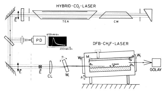
Figure 1 Experimental arrangement of grazing-incidence 496  $\mu m$  CH<sub>3</sub>F laser.
