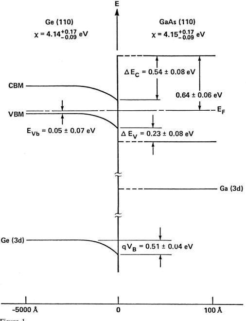
Figure 1 Experimental results for the band parameters across the Ge(110)/GaAs interface. The horizontal axis is in the thousands of angstroms on the substrate side of the junction, while the overlayer is presented in tenths of angstroms only.
