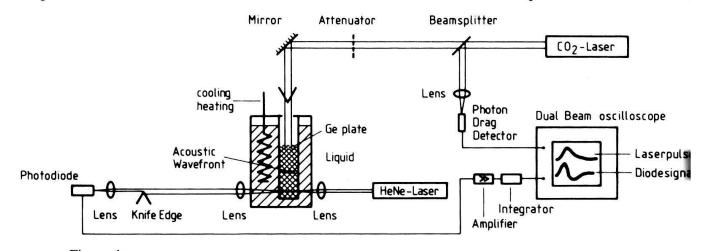
Figure 1 Schematic diagram of the experimental arrangement.
