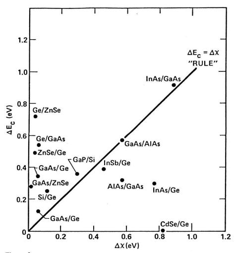
Figure 2 Conduction band discontinuity  $\Delta E_c$  measured by core level photoemission spectroscopy plotted as a function of electron affinity. The band gaps and the electron affinities are from Ref. 17. The substrate semiconductor is written first and the overlayer written second.
