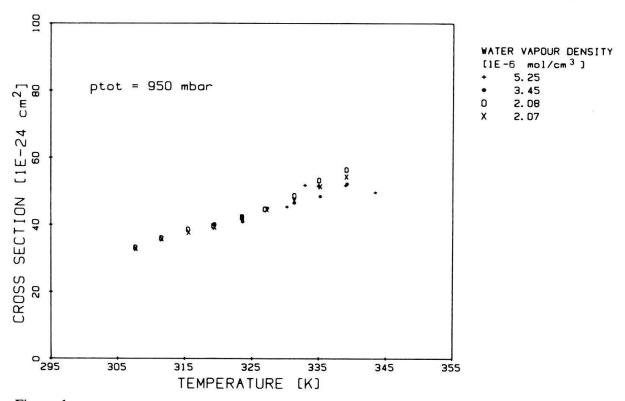
Figure 1 Absorption cross section of water vapor vs. temperature at the  $10\,\mathrm{R}(20)\,\mathrm{CO}_2$  laser transition. Experimental data corresponding to four different vapor densities are plotted.
