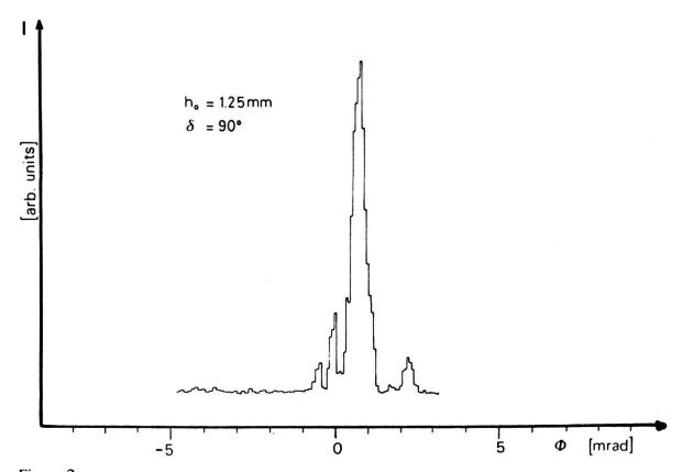
Figure 2 Example of resonant 496 µm laser emission.
