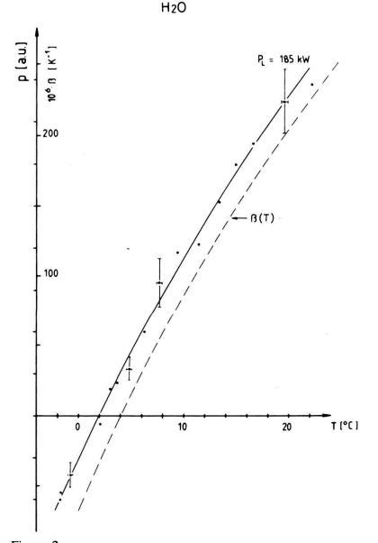
Figure 2 Temperature dependence of the observed peak pressure p in distilled water compared to that of the thermal expansion coefficient  $\beta$ .
