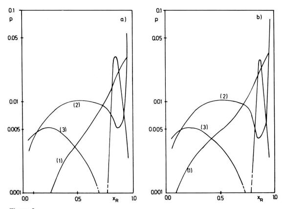
Figure 3 The absorbed power is plotted as a function of the position  $x_R$  of the resonant surface for (1) k = 0.01, (2) k = 1.01 and (3) k = 2.01. In all cases, m = +1. The results shown are for MHD standard conditions (a) without and (b) with gravity. The scanning step used for  $x_R$  is  $\Delta x_R = 0.05$ .
