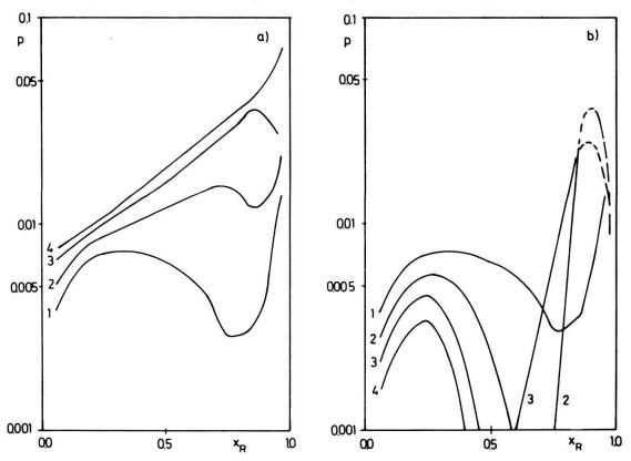
Figure 5 The absorbed power is plotted as a function of the position of the resonant surface for  $\omega/\omega_{ci} = 0.0, 0.2, 0.4, 0.6$  (curves labelled 1, 2, 3, 4). In (a), k = -1.5, m = -1 and in (b), k = +1.5, m = +1. Standard conditions without gravity are used, and  $\Delta x_R = 0.05$ .
