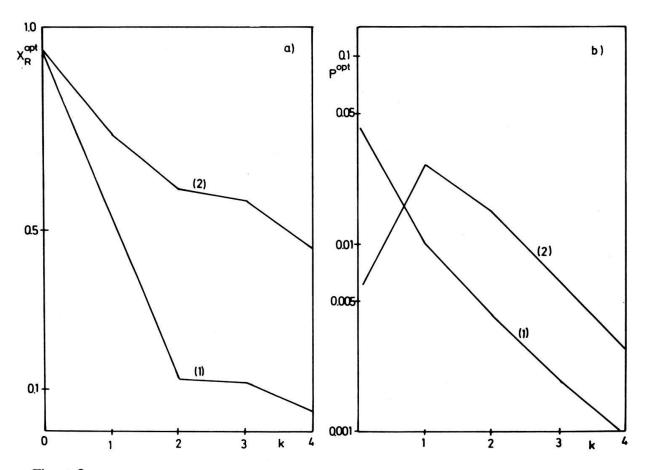
Figure 2 The position of optimal resonance layer (a) and optimal power (b) is plotted as a function of the axial wavenumber k for m = +1. Curve (1) refers to standard MHD conditions; whereas, curve (2) refers to the currentless, i.e., shearless case. The gravity field is zero in both cases.
