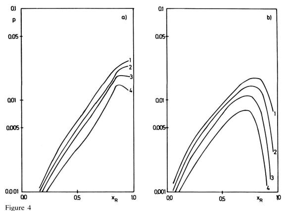
The absorbed power is plotted as a function of the position,  $x_R$ , of the resonant surface for  $\omega/\omega_{ci} = 0.0$ , 0.2, 0.4, 0.6 (curves labelled 1, 2, 3, 4). In all cases gravity was not included and m = +1. In (a) k = 0.02, and in (b) k = 0.5. In both cases  $\Delta x_R = 0.05$ .
